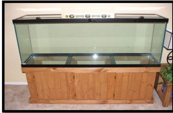
Figure 11: Fish Tank for Thrust and Power Testing
